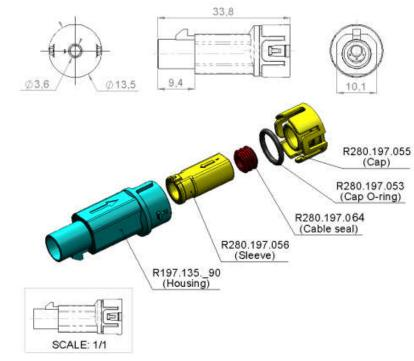
To obtain the complete P/N please fill in the blank "\_" with the coding letter Coding Z is shown for information
